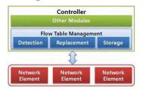
Figure 5 Flow Table Management's Architecture.
