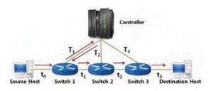
Figure 4 Controller replaces flow entries.
